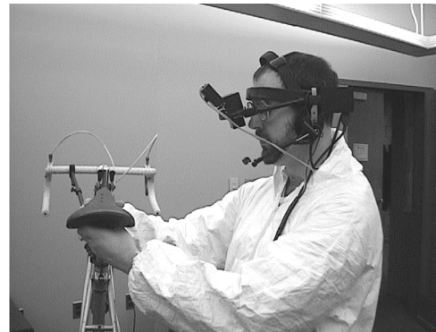
Figure 2: Worker wearing collaborative system.
