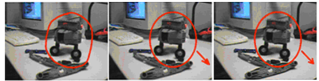
Figure 4. Remote gesture recognition in a robot building task. A freehand oval and arrow (left, center) have been regularized by the recognition component (right)
